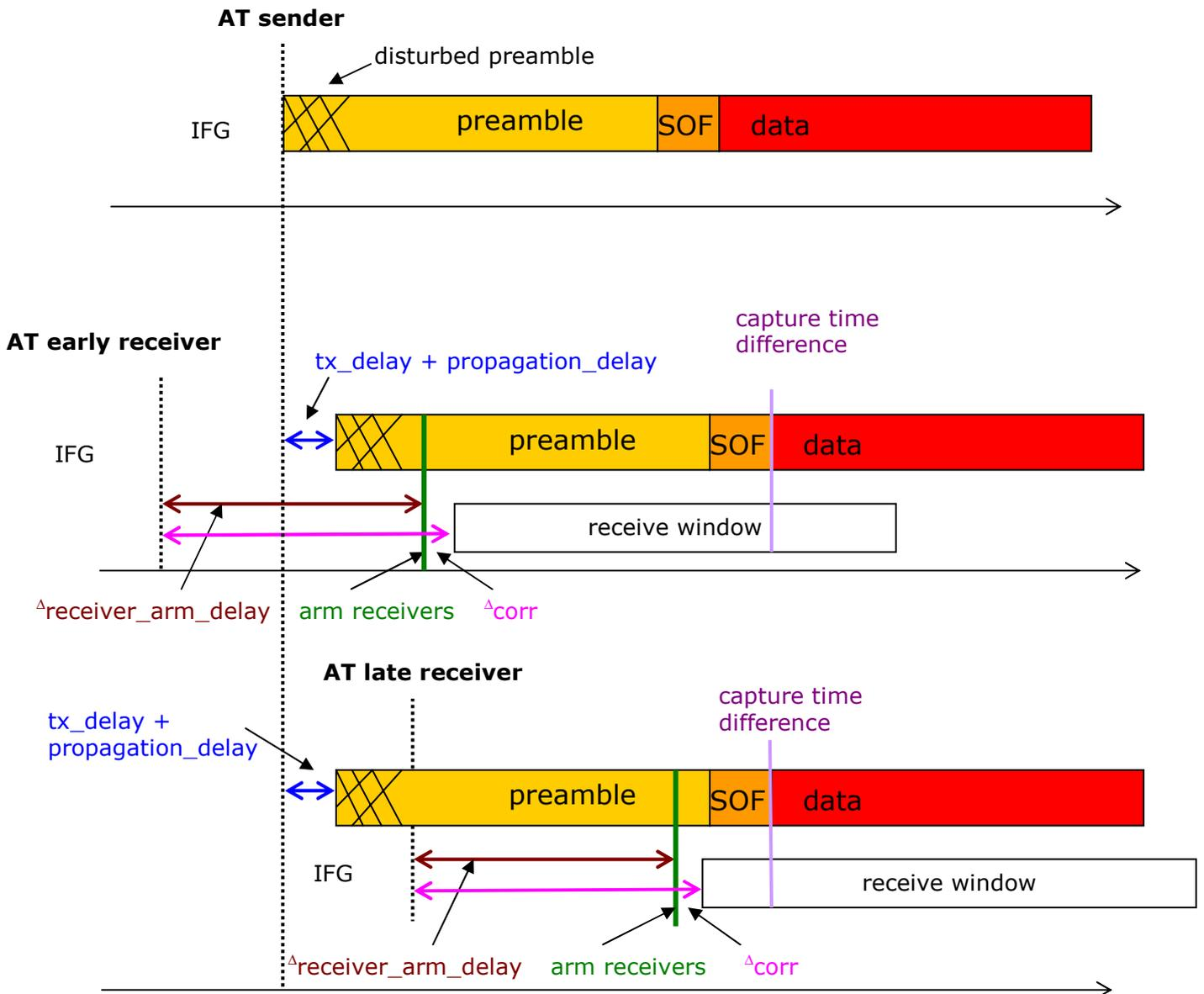
As shown in the figure above, the  $\Delta_{\text{receiver\_arm\_delay}}$  must end *before the receive window* is opened (AT +  $\Delta_{\text{corr}}$ ).
