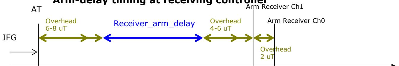
**Arm-delay timing example (Manchester encoding ) for an early and a late receiver with receiver protocol version  $\geq 2.00$**
