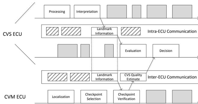
Fig. 5. Overview of CVS/CVM tasks, task to CPU/ECU assignment, and intra-ECU inter-ECU communication
