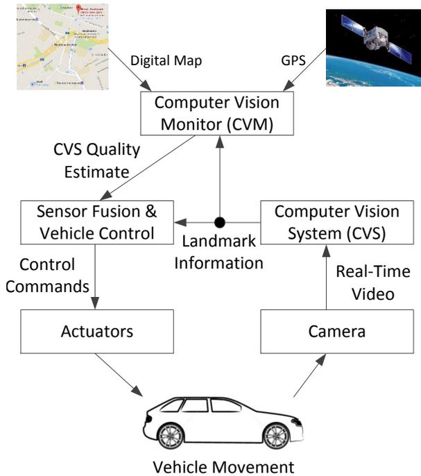
Fig. 1. Computer vision monitor - an example for infrastructure support
