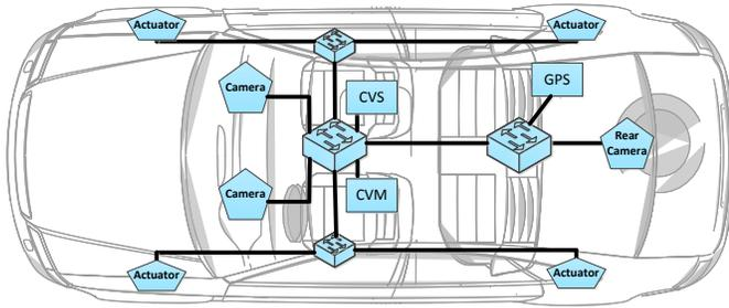
Fig. 4. Idealized setup of an in-vehicle computer-vision system and computer-vision monitor (redundancy levels are not depicted)
