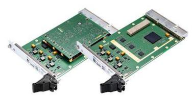
Caption: First electronic equipment for module of the NASA Gateway: The <sup>TTE</sup>Switch Space 3U cPCI and <sup>TTE</sup>End System Space 3U cPCI are among the first form-fit and functional equipment delivered for the Gateway projects in July. (© TTTech Computertechnik AG) Download high resolution image: <u>https://www.tttech.com/wp-content/uploads/RUAG\_print\_01-notext.jpg</u>
