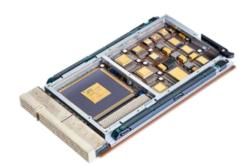
**Caption**: TTEEnd System Space 3U cPCI, one of the components of TTTech Aerospace's TTEthernet network and computing platform (Copyright: TTTech Computertechnik AG)
