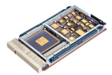
**Caption:** TTTech Aerospace's modular network equipment, designed and manufactured in cooperation with RUAG Space incorporates switches, end systems, software elements and network configuration tools. It can be seamlessly integrated in different configurations into a standard hosting unit. Pictured: TTESwitch Space 3U cPCI. (Copyright: TTTech Computertechnik AG)
