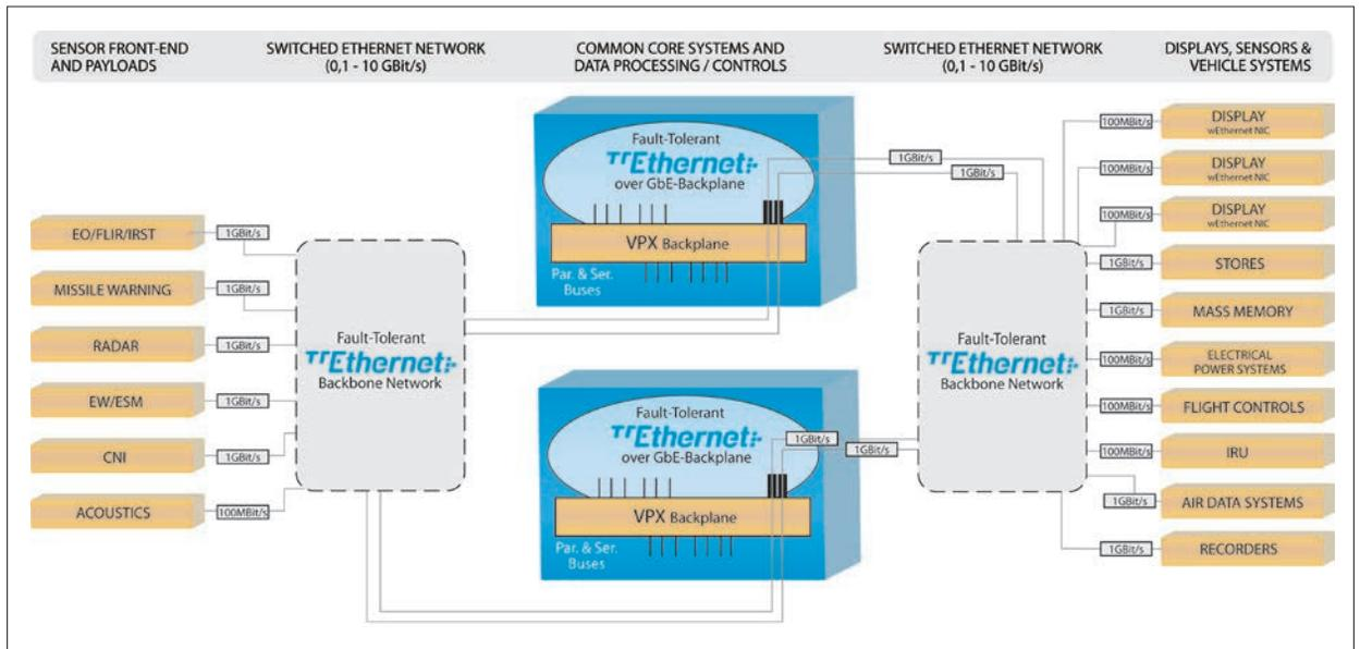
Deterministic Ethernet as backplane/backbone network enables design of advanced integrated systems and architectures.
