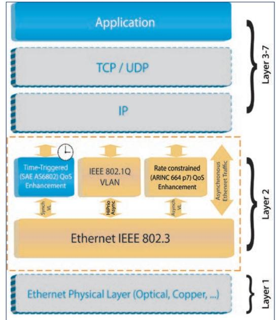
**TT**Ethernet switch provides time-triggered (synchronous), rate-constrained and regular Ethernet traffic class.
